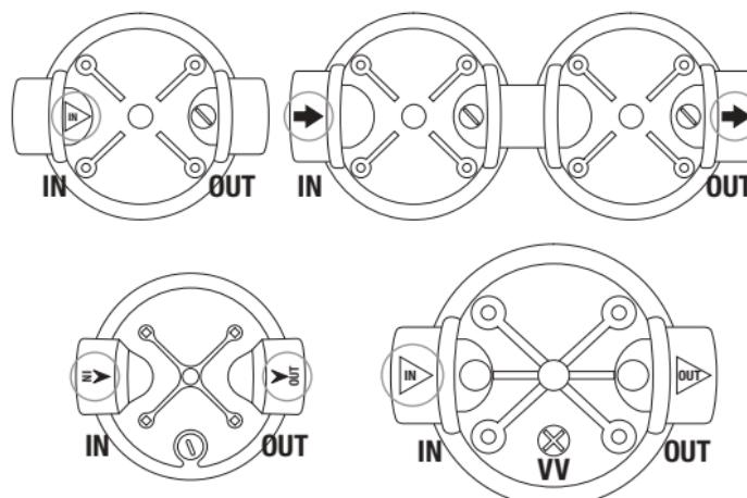
Installation of gauges and/or drain kit for models with such accessories: M models (with gauges) S (with drain kit) and SM (with drain kit and gauges)
