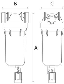
Max working pressure \_\_\_\_\_ 8,3 bar (120 psi)
