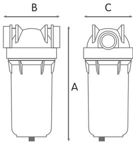
Max working pressure \_\_\_\_\_ 8,3 bar (120 psi)
